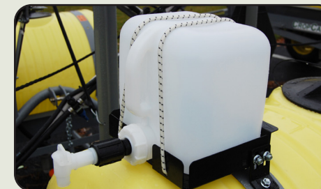
Fresh water safety tank
